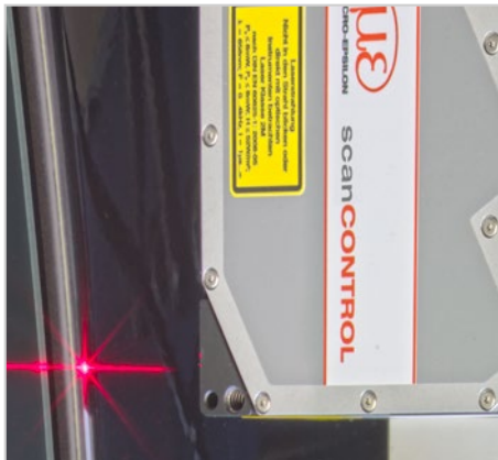
Gap measurement on car bodies
