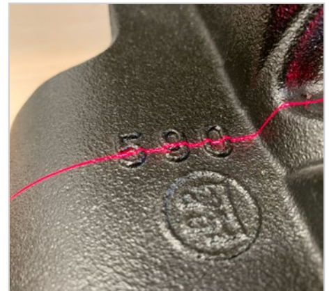
Text recognition on the cast part
