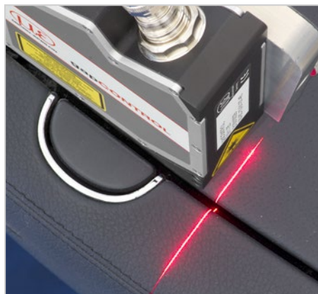
Distance measurement at the center console
