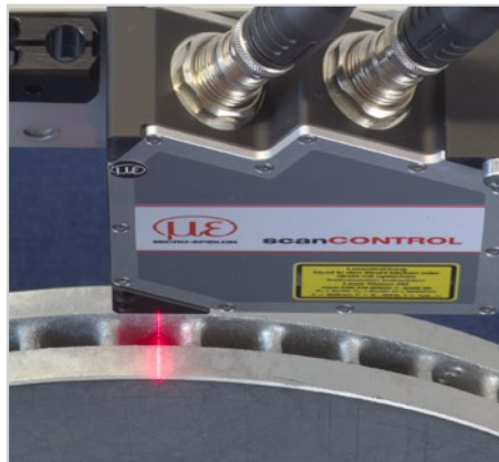
Profile measurement of the brake disc
