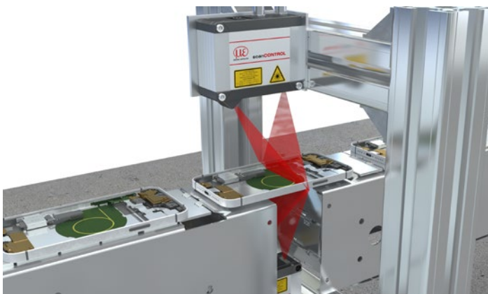
Thickness of smartphone carrier plates
