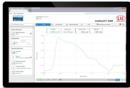
Settings are made via the web interface. For thickness measurements, materials are stored in an expandable materials database.
