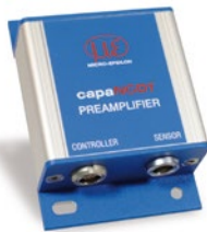
CPM6011 External pre-amplifier for standard measurements
