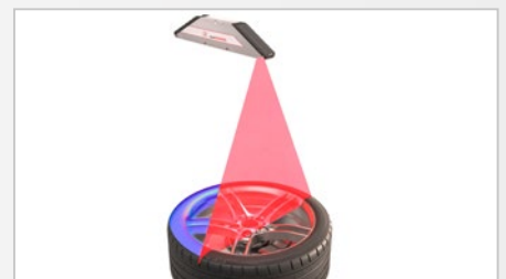
Inline 3D inspection of tire geometry
