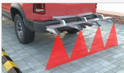
Detection of the road surface profile
