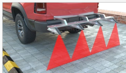
Detection of the road surface profile
