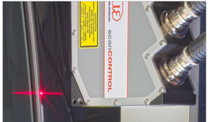
Gap measurement on car bodies
