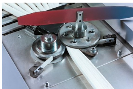
Inline yarn thickness measurement
