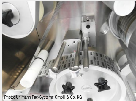
Foreign body detection in blister packs
