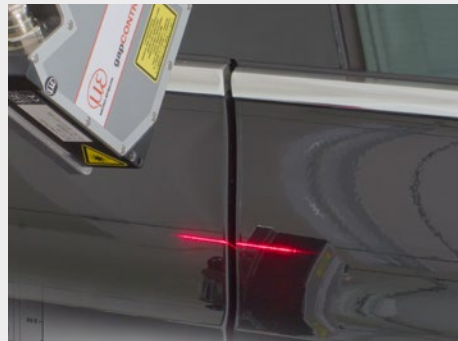
Gap and flushness measurement on bodywork parts
