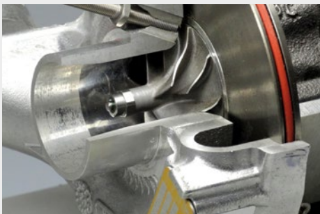
Rotational speed measurement of turbochargers
