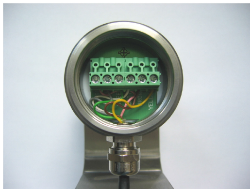
Fig. 15 View on terminal block with sensor cables
