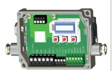
Fig. 10 Opened controller CTM-4 with terminal connections
