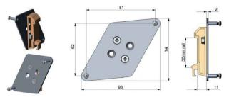
Fig. 47 Rail mount adapter for controller [TM-RAIL-CT]
