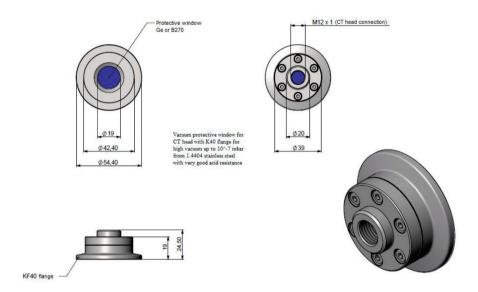
KF40 flange (TM-KF40GE-CT) with Ge window or TM-KF40B270-CT for CTM-1, CTM2, CTM3 with B270 window
