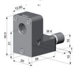
Fig. 41 Laminar air purge collar [TM-AP-CT]
