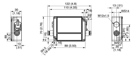
Fig. 7 Dimensional drawing controller CTM-4, dimensions in mm (inches), not to scale
