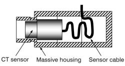
Fig. 55 Massive housing
