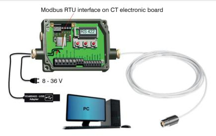
Fig. 23 Installation Modbus RTU interface on thermoMETER CT electronic board
