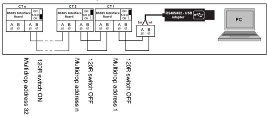
Fig. 19 Pin assignment RS485
