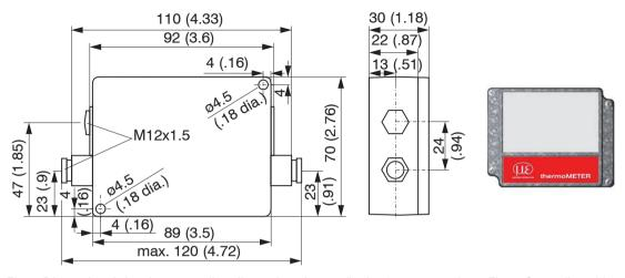
Fig. 5 Dimensional drawing controller, dimensions in mm (inches), not to scale
