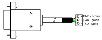
Fig. 18 Pin assignment RS232
