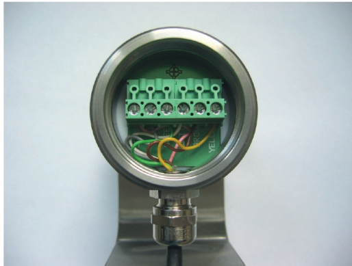
Fig. 15 View on terminal block with sensor cables
