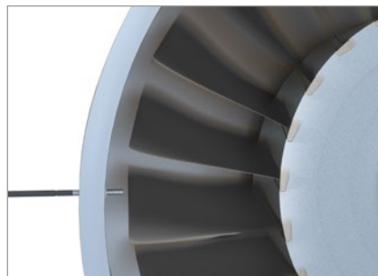
Radial installation: measurement in turbines
