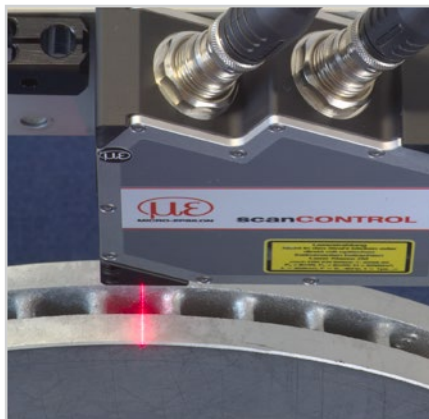
Profile measurement of the brake disc
