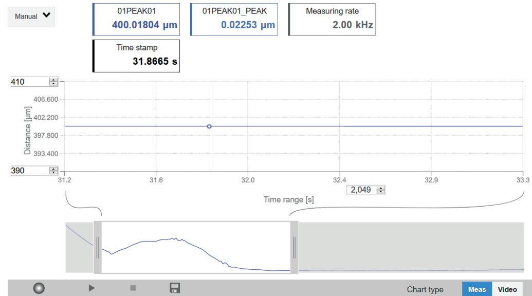
Fig. 76 Offline analysis of measured thickness results based on a one-sided thickness measurement
